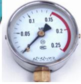
**2. Checking the Pool Filter pressure gauge** to see if it needs a backwash.
