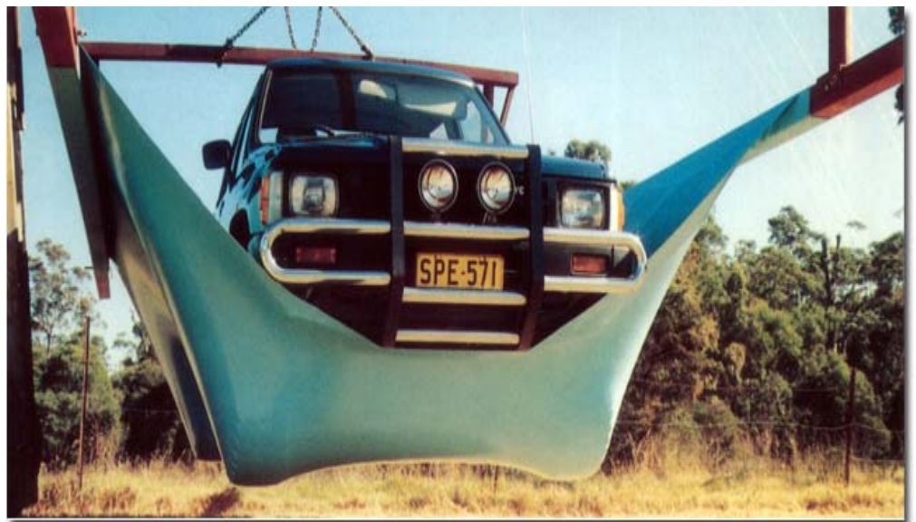
The famous Landcruiser Lift using NYLEX swimming pool liner material
